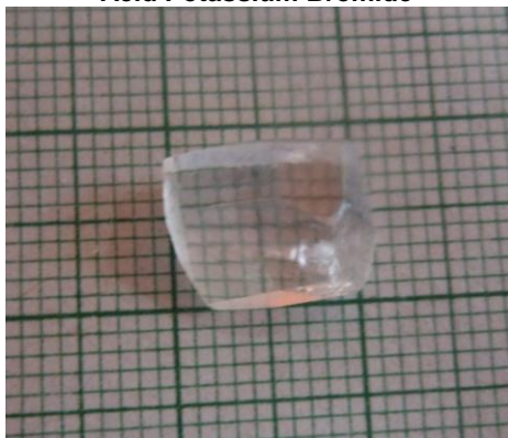
Figure 1 Grown crystal of Urea Doped Tartaric Acid Potassium Bromide
